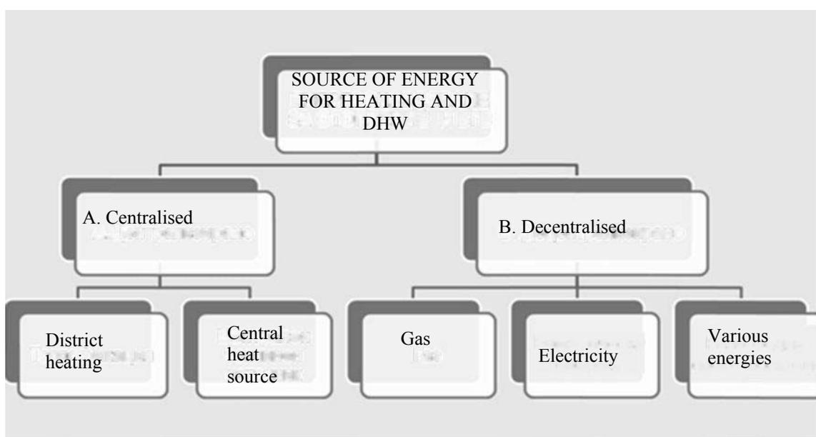
Figure 1.2.2-7 High-level classification<sup>3</sup> of buildings by type of heat-supply system
